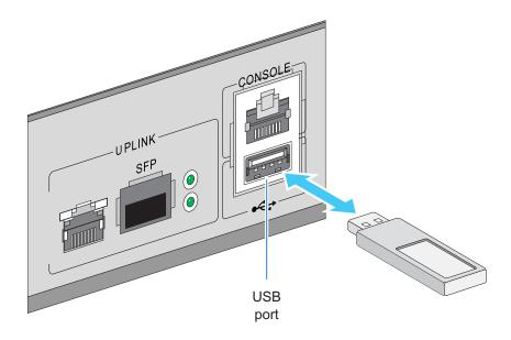
The Brocade Mobility RFS4000 Controller contains one USB port for connecting USB flash storage devices to the controller. The controller can use the USB flash storage device for file transfers and firmware updates. Follow the setup instructions below to connect the devices to the controller and then access those devices through the Web UI or Command Line Interface.
