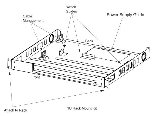
2. Place the power supply unit in the rack mount tray in the space provided.
